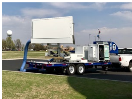
Dual-pol phased array prototype completed
