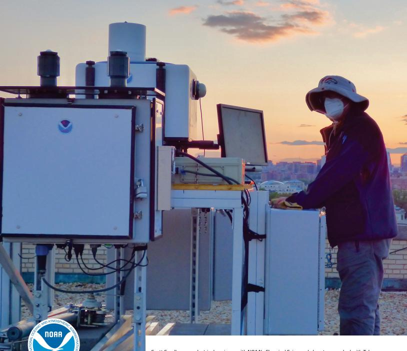
Scott Sandberg, an electrical engineer with NOAA's Chemical Sciences Laboratory, worked with Tyler Boyle of NIST to install a Doppler lidar instrument on April 16, 2021, on top of the Department of Commerce's Herbert Clark Hoover Building in Washington, D.C. for a research project studying urban greenhouse gas emissions. Credit NOAA's Scott Sandberg and NIST's Tyler Boyle
